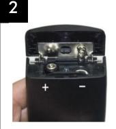
Install 2 AAA batteries. Make sure the + and symbols on the metal hinge of the battery compartment correspond with the + and - end of each battery.
