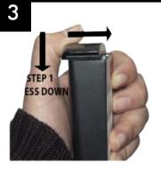
With the keypad facing away from you, close the cover by gently pressing it down (STEP 1) and sliding it until it aligns with the front (keypad) of the device (STEP 2).
